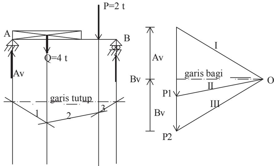
$$\begin{aligned} Q &= q \cdot l' \\ &= 1 \text{ t/m} \cdot 4\text{m} \\ &= 4\text{t} \end{aligned}$$
