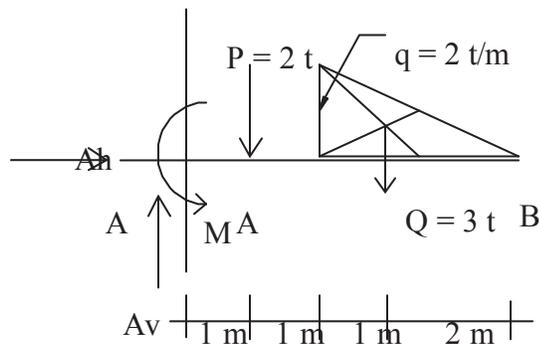
$$\begin{aligned} \text{Besar } Q &= 1/2q \cdot l \\ &= 1/2 \cdot 2\text{t/m} \cdot 3\text{m} \\ &= 3\text{t} \end{aligned}$$
