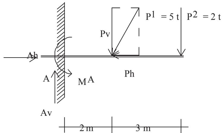
$$\begin{aligned} P_v &= P_1 \sin 60^\circ \\ &= 5t \cdot 0,866 \\ &= 4,33t \end{aligned}$$
