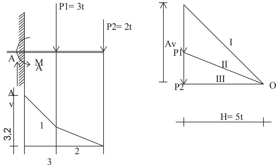
Besar reaksi-reaksi tumpuannya :  $AV = 5 \text{ cm} \times \frac{1 \text{ t}}{1 \text{ cm}} = 5 \text{ t}$
