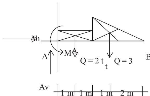
$$\begin{aligned} \text{Besarnya } Q_1 &= q \cdot l \\ &= 1\text{t/m} \cdot 2\text{m} \\ &= 2\text{t} \end{aligned}$$
