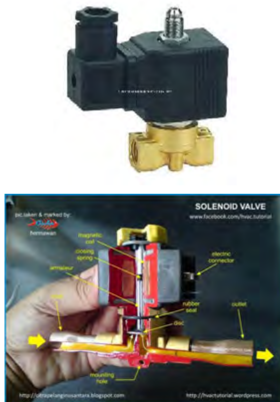
Gambar 2. 41 Solenoid Valve
