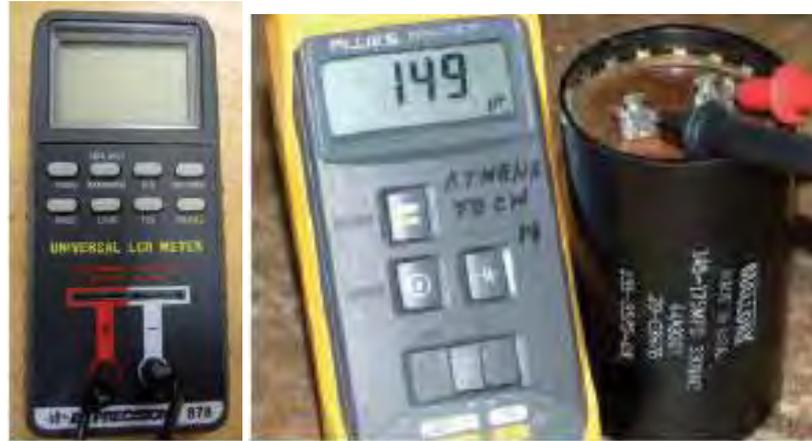
Gambar 5.8 Capacitor Analyser
