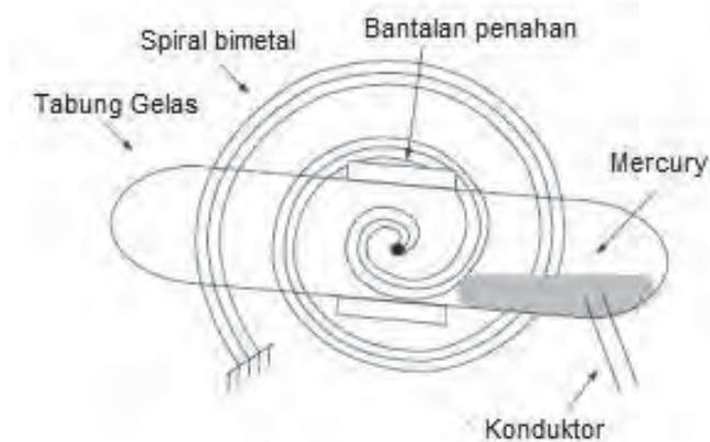
**Gambar 1.19 Mercury switch**
