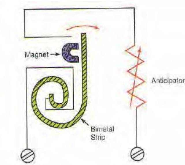
Gambar 3 .12 Skematik diagram Pengawatan Heating Thermostat
