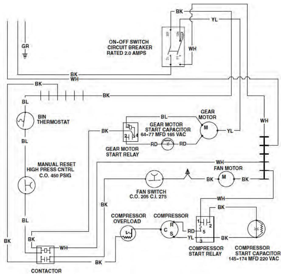
Gambar 4.12 Diagram Ladder System Control Refrigerasi Komersial
