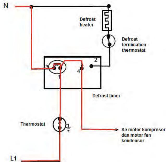
Gambar 4.26 Tipikal Rangkaian Defrost Cumulative Run
