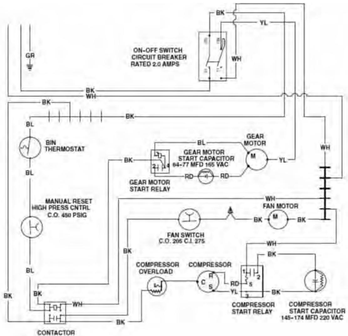
Gambar 5.18 Diagram Ladder system control Refrigerasi komersial
