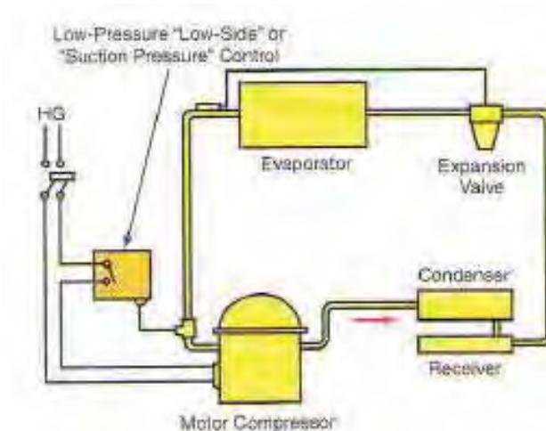
Gambar 4.17 Skematik Low-pressure Motor Control
