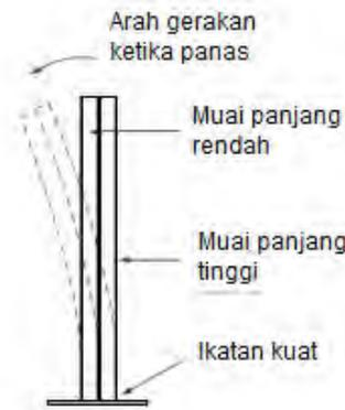
**Gambar 1.18 Bimetal Strip Switch**
