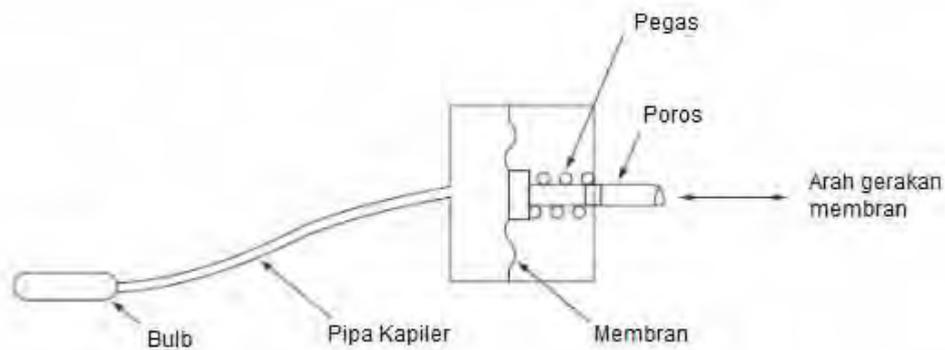
**Gambar 1.20 Bulb & Capillary switch**
