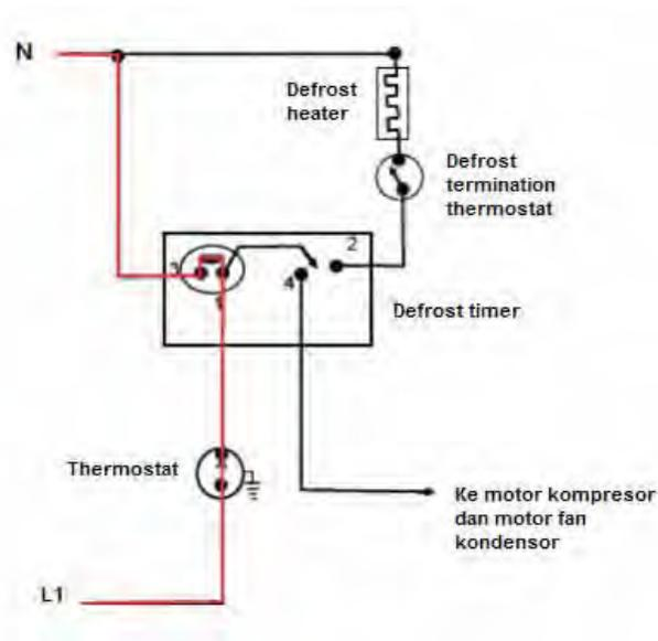
Gambar 4.25 Tipikal Rangkaian Defrost Cumulative Run
