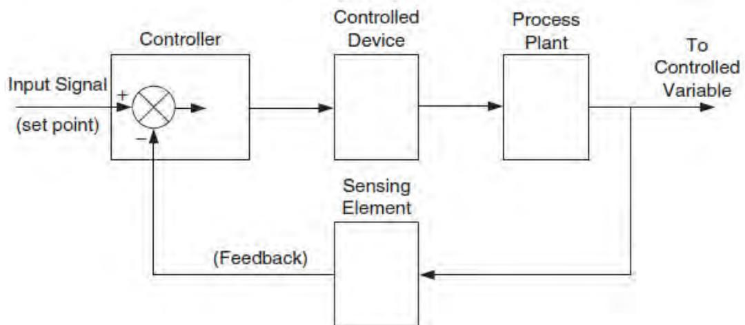
**Gambar 1.2 Diagram Control Loop**
