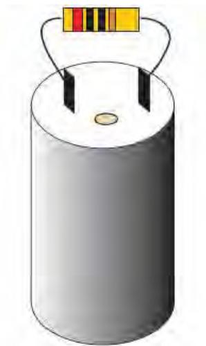
Gambar 5.5 Bleed Resistor Pada Kapasitor
