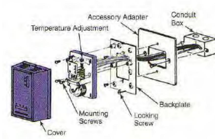
Gambar 3.6 Tipikal Line-voltage Thermostat
